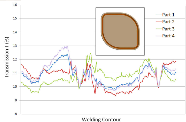
Fig. 1: Component dependent transmission profiles along the welding contour of a typical GFK automotive part
