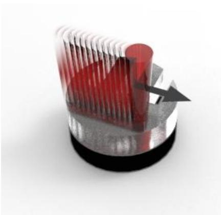
*Figure: Principle of quasi-simultaneous welding*
