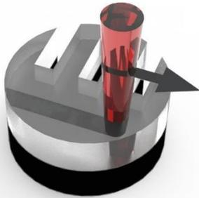
*Figure: Principle of contour welding*
